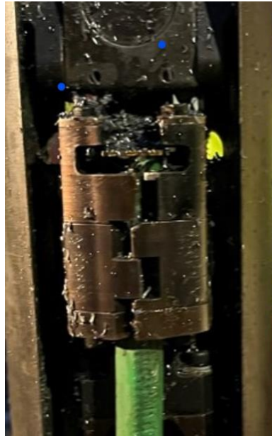
Gripper locked onto control line
