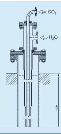
Design of system with separate injection and sparger to mix in well
