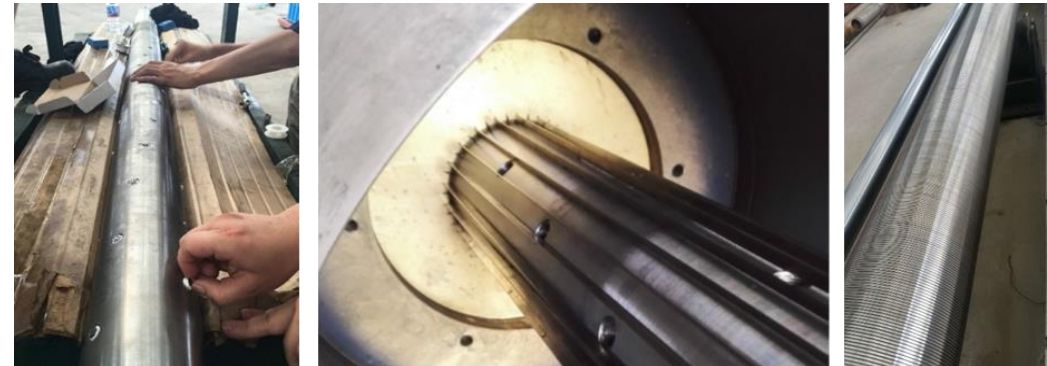
Valve insertion, screen wrapping and CFD final product
