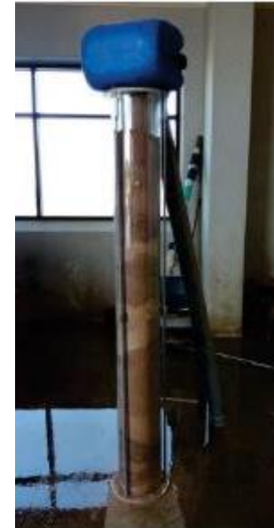
Pic 2 Annulus filled with settled Barite
