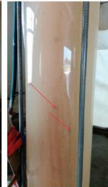
Pic 5 Clean out finished, perforations are now visible.
