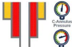
Sustained Casing Pressure
