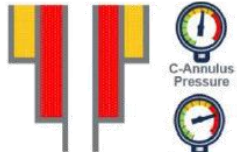
Sustained Casing Pressure
