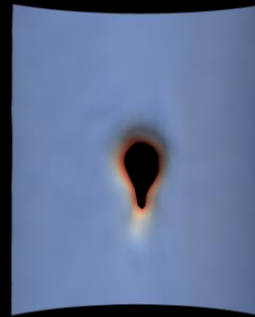
Geometric Quantification of Eroded Perforation
