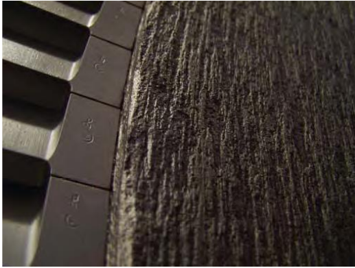
Severe wheel erosion
