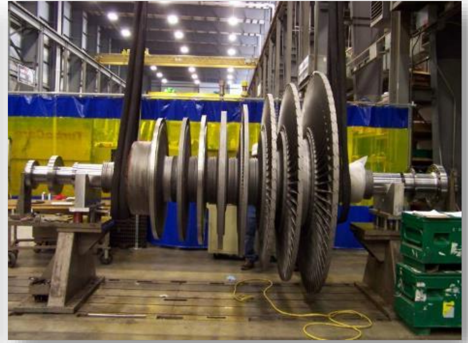
1st & 3rd stage reblading completed
