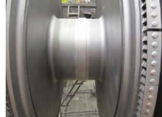
Finished photo of wheels machined and Inconel inlay in shaft seal area
